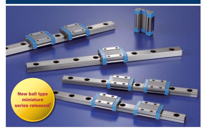
MLV series is a super small-size linear motion rolling guide produced by original small sizing technology. Thanks to the structure with two rows of balls to contact with the way at four points, stable accuracy and rigidity can be achieved even in applications where load has variable direction and size or complex load is applied, despite its very small body and light weight.
